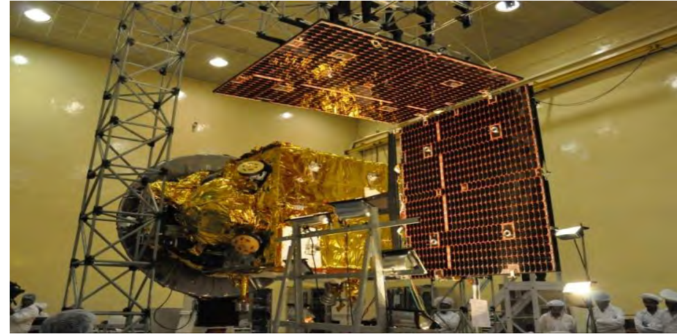
Solar Panel Deployment Testing
