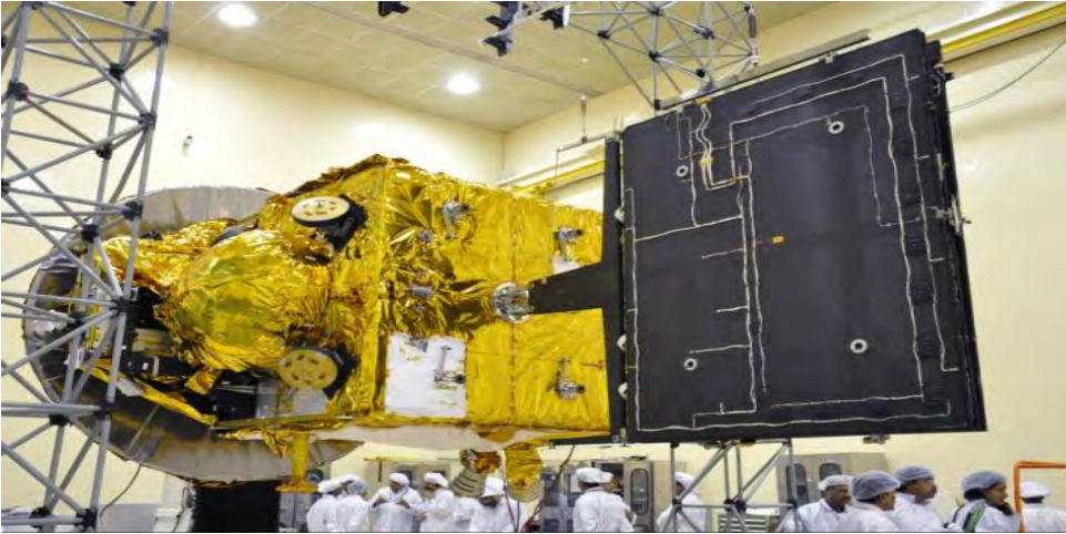
Solar Panel Deployment Testing
