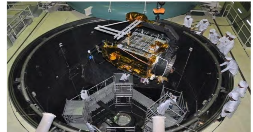
Loading into Thermovac Chamber
