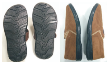
Complete footwear fabricated using the injection molded PU-nanofiller composite sole
